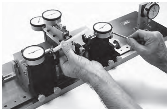
Inserting ceramic cylinder in gage to check squareness and parallelism of ends, longitudinal bow and out-of-roundness
