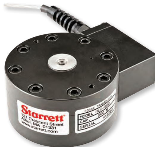
MLC low-profile load cell sensor Load measurement accuracy of \pm 0.5\% of reading down to 1/100 of sensor capacity may be achieved.
