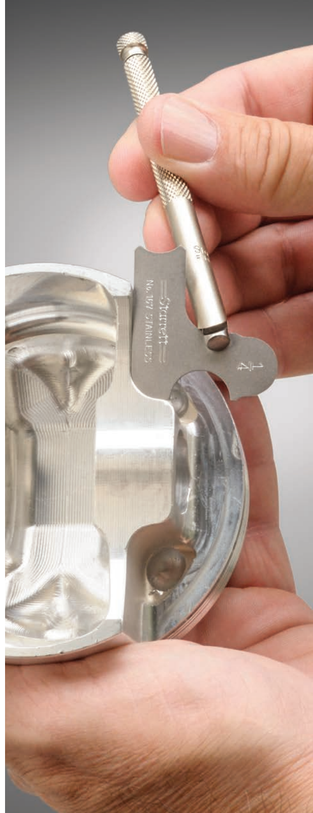
Gaging radii using gage with holder
