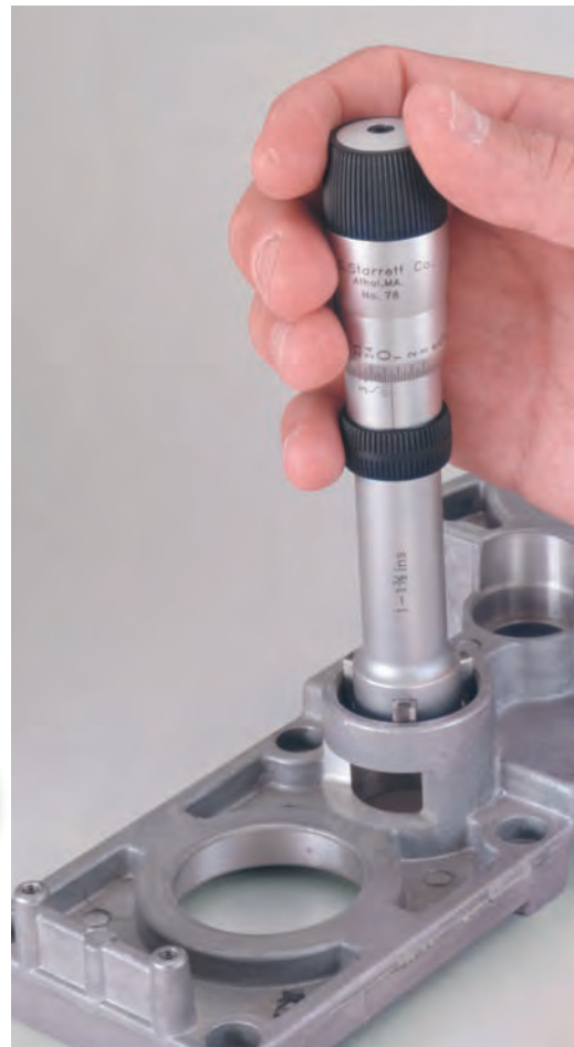
78XTZ-138 Measuring a bore
