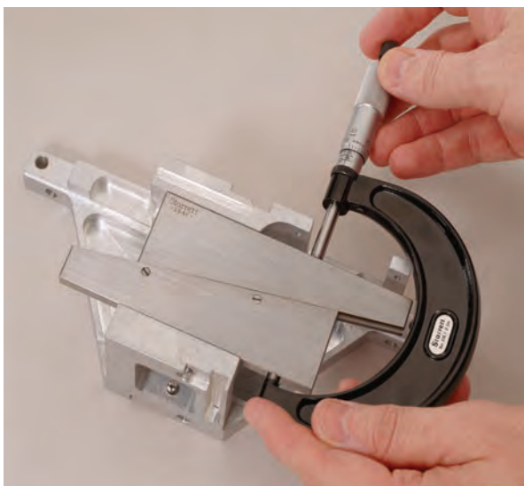
Checking inside measurement of slot with parallel and outside micrometer
