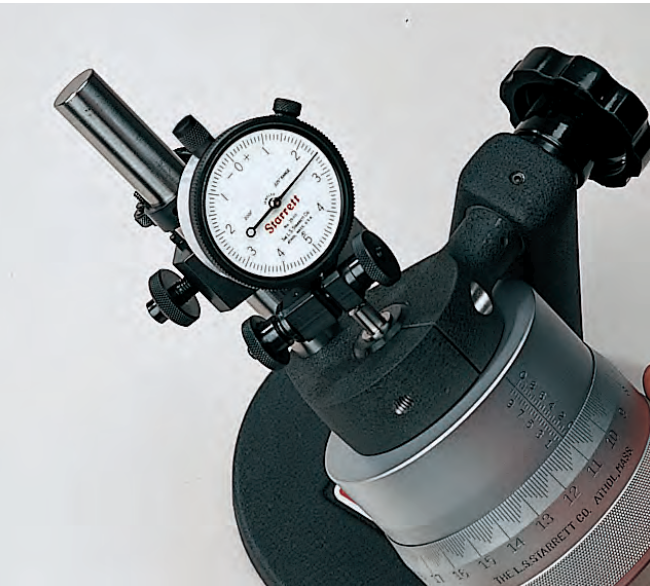
Checking AGD dial indicator
